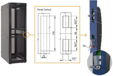
TANlock options come with all required hardware for mounting to an Eaton enclosure or other universal cutout enclosure doors. For required dimensions and installation instructions, consult the user guide found at Eaton.com/TANlock.
